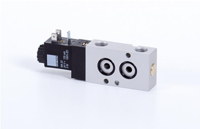
The picture displays an **MNH 310 701**, which is a **3/2-way** single solenoid NAMUR-valve. It is used to control a single-acting actuator.
